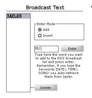
order to broadcast certain message through the RDS go to the BROADCAST TEXT frame. Type a word in the blank frame and then click "enter" or the use "enter" button of your kevboard. After that the word will be added first in the list on the right. Carry on with this procedure adding all the words you need. You
